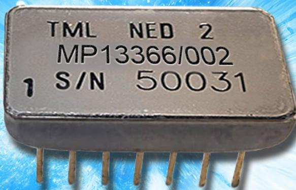
Micross continues to offer our First Generation (Technograph) NED for legacy or new equipment requiring cost-effective nuclear protection. The First Generation NED provides an output in response to gamma radiation, that is used to protect sensitive electronic circuitry.
